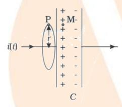
Case 2: Maxwell considered a surface, like a box with its lid open and applied the Ampere's circuital law;
