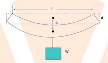
A bar of length 1, breadth b, and depth d, when loaded at the centre by a load W sinks by an amount given by  $\delta = \frac{WI^3}{\left(4bd^3Y\right)}$
