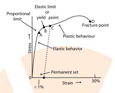
Above graph shows the stress-strain curve for a metal wire which is gradually being loaded.
