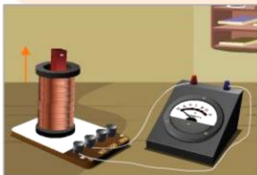
The North Pole of the Magnet is Moved out of the Coil of Wire
