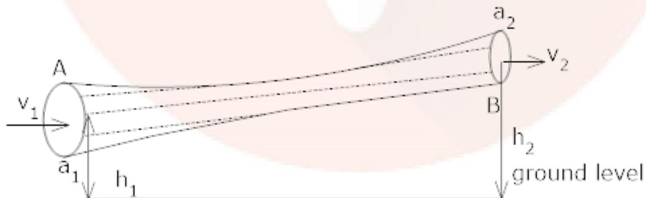
$p_1$  = Pressure applied on liquid at A
